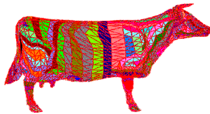
Figure 5: Applying stripification to a cow mesh [55]. Different colors represent different triangle strips. ( http://www.cosy.sbg.ac.at/~held/projects/strips/strips.html )
